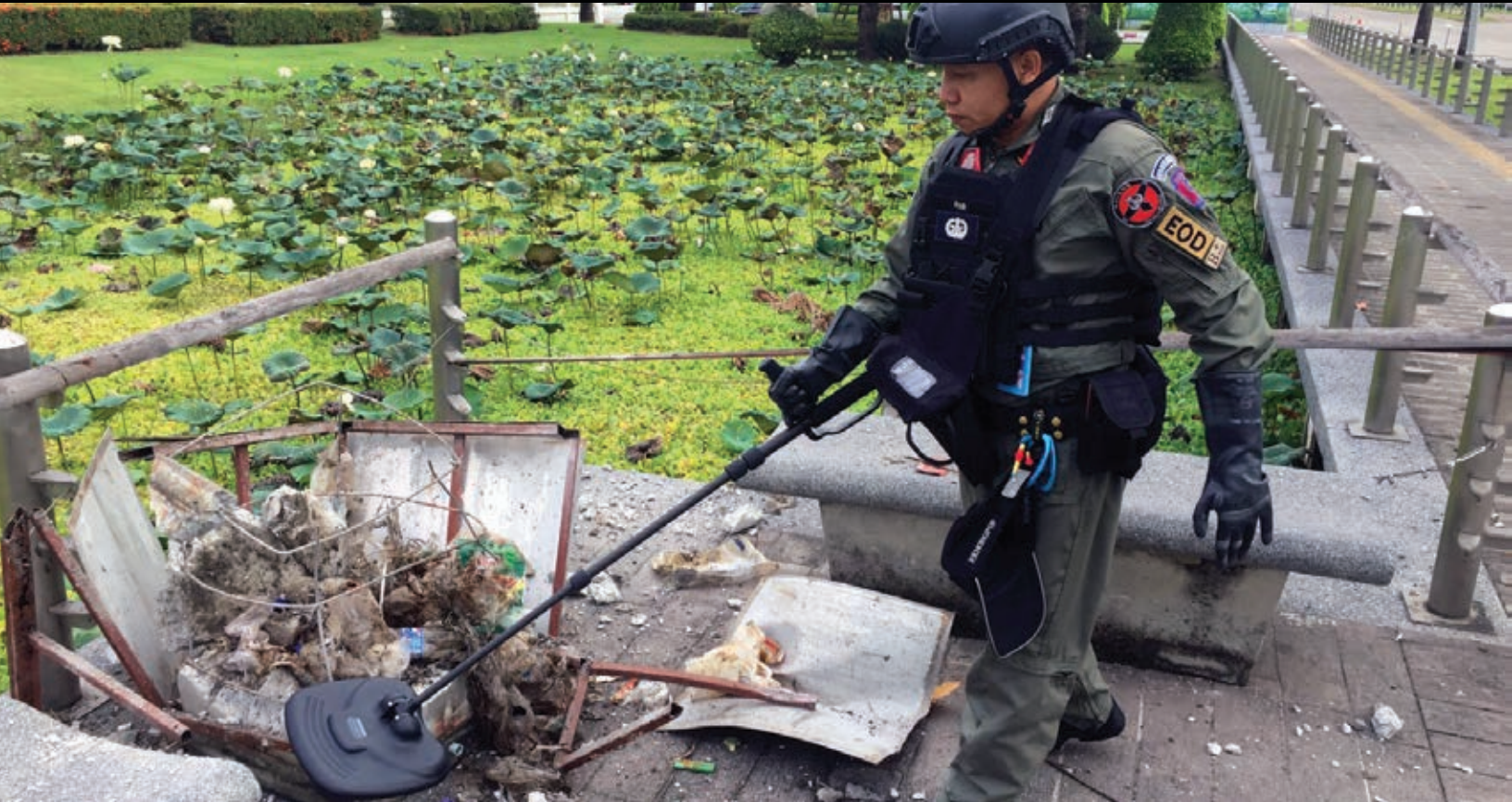
An ATA-trained bomb tech with the Royal Thai Police Metropolitan Police Bureau uses a nonlinear junction detector to scan for components of a detonated IED at a blast site in Bangkok on August 2, 2019. (Photo courtesy of Royal Thai Police)
